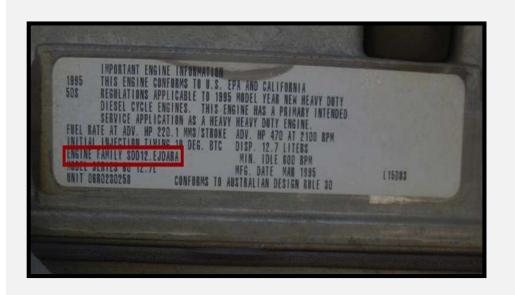
Required on all 1974 or newer diesel powered heavy-duty commercial engines operating in CA
