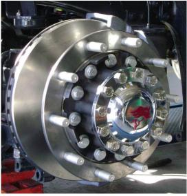
The weight benefit afforded by air disc brakes depends upon the overall wheel-end components chosen as part of the package.
