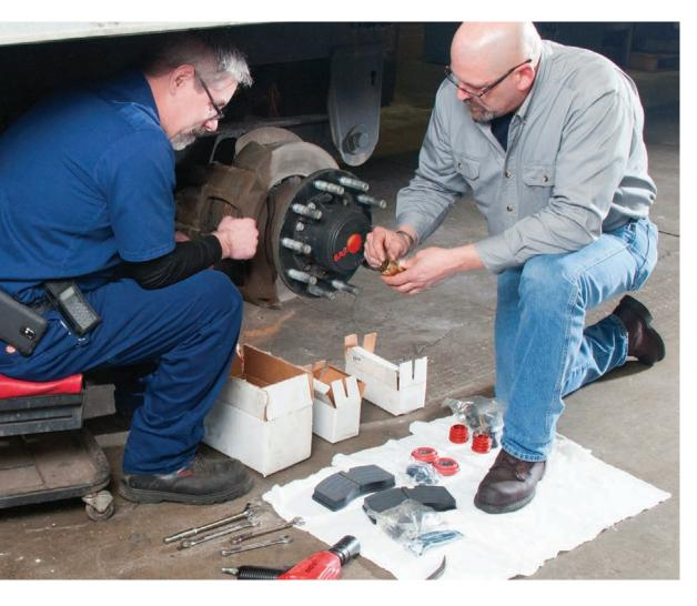
Disc brakes are about a \$1,200-per-axle premium over drums but offer reduced maintenance costs if they are maintained correctly.
