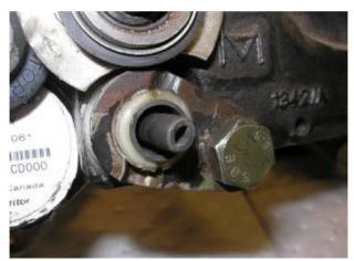
Fig 8 Adaptor and connector fitted
