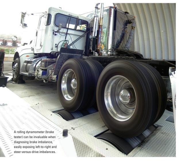
Diagnosing and correcting brake imbalance issues is critical for vehicle performance and safety over the road.
