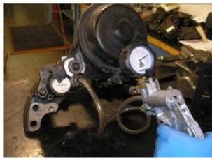
Fig 9 Vacuum tester in position
