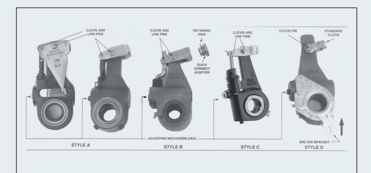
Fig. 2: Self-Adjusting Brake Adjuster Types
