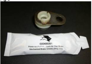
Fig 6 Vacuum test adapter plug (MST1504) and grease (68966091)
