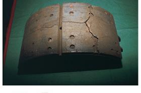
Cracked linings likely were loose on the shoe. This is caused by a shoe that's out of arc, rust buildup on the shoe surface or improper riveting.
