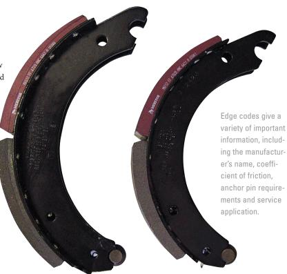
labeled on the edge code of a friction lining material, it is a reference and not indicative of the performance of that particular friction. It's very important for technicians to bear that in mind when comparing edge codes."
