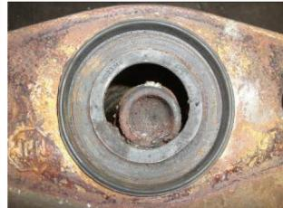
Fig 10 Corrosion on ball end of actuator and liner part of seal
